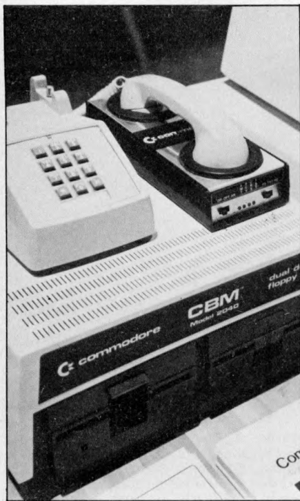
Left: Commodore's acoustic modem will let PETs converse over long distance telephone. Below: Common Sense security system — PET monitors alarm and displays security zones on screen.
